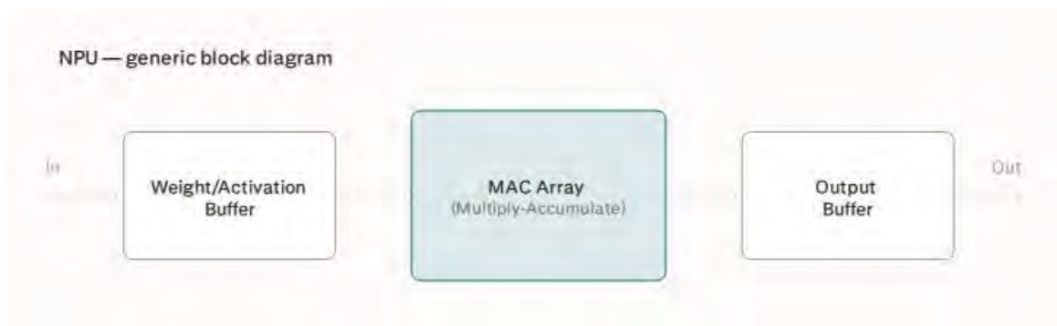
Figure 8. NPU generalized block diagram
